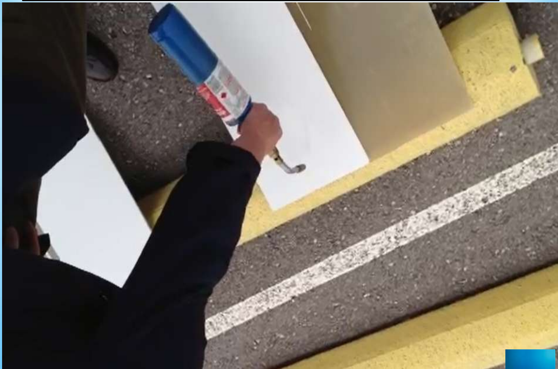
30 sec video of fire char formation on gel coat with propane blow torch
