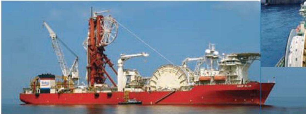
Deep Blue: Technip's deepwater pipelay vessel
