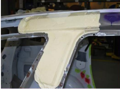
Cavity Filling – Elastoflex W ®
