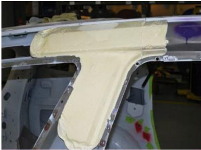
Cavity Filling – Elastoflex W ®
