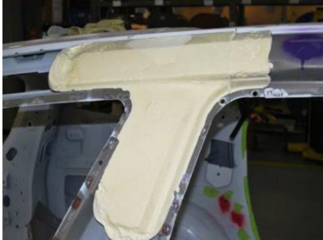
Cavity Filling – Elastoflex W ®
