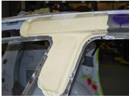
Cavity Filling – Elastoflex W ®
