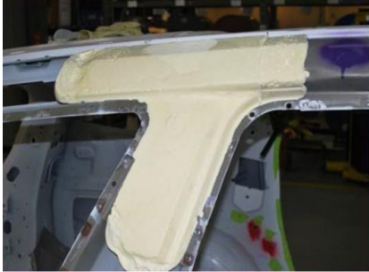
Cavity Filling – Elastoflex W ®
