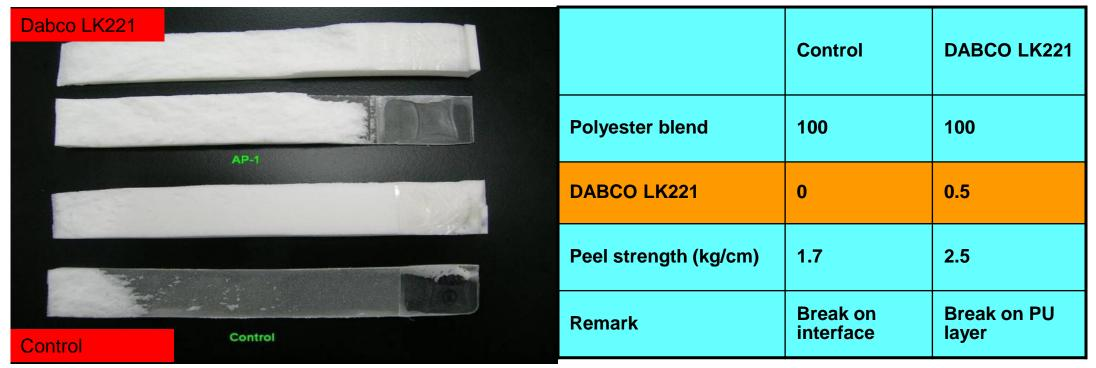
Adhesion test between PU and TPU
