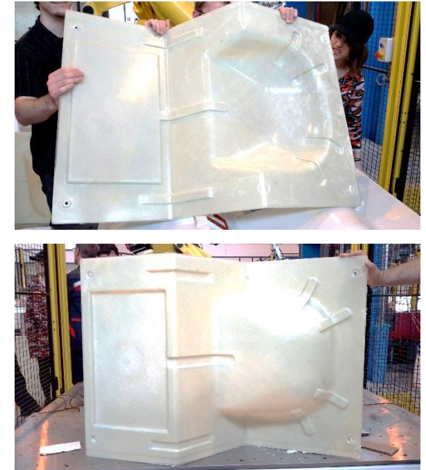
Glass fiber reinforced Elium® resin demo part made on Fast-RTM pilot line
