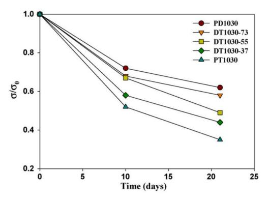
Higher content of ester groups in polyurethane structure inhibited the loss of the mechanical properties after hydrolitic degradation
