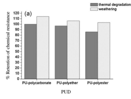
Polyurethanes made with polycarbonate diol showed higher retention of chemical resistance both after thermal degradation and upon weathering
