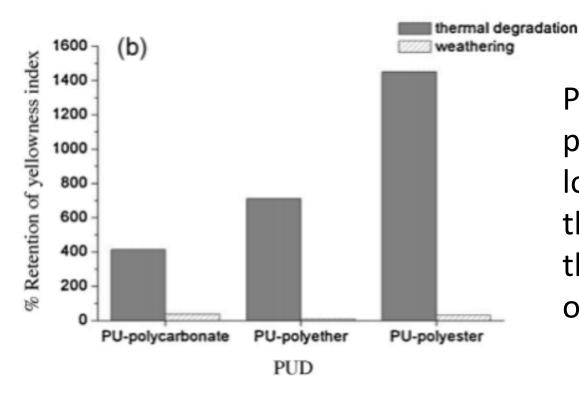
Polyurethanes made with polycarbonate diol showed lower yellowness after thermal degradation than those made with polyether or polyester
