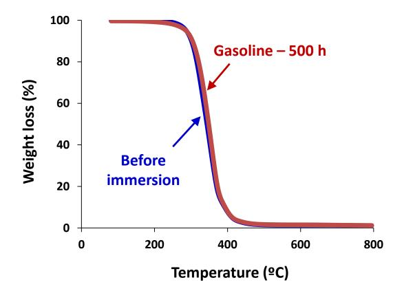
Thermal stability of PU sealant made with polycarbonate diol Eternacoll® doesn't change after immersion in gasoline
