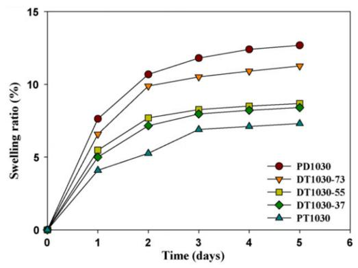
Higher content of ester groups in polyurethane structure increased the swelling resistance in hot water of the PU sealant
